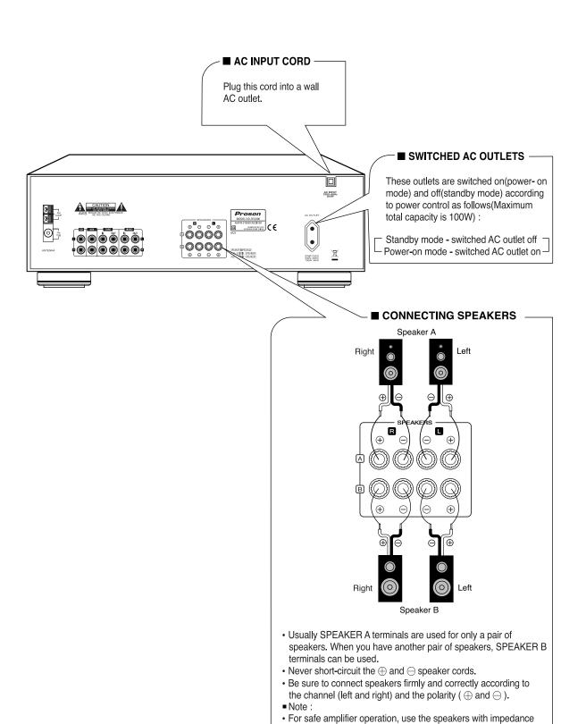
of over 8  $\varOmega$  when you use only SPEAKER A or B terminals and use the speakers with impedance of over 16  $\varOmega$  when you use
